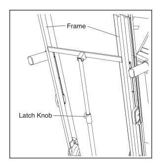
2. Hold the metal frame firmly with both hands and lower it to the floor. CAUTION: Do not grip only the plastic foot rails or drop the frame to the floor. Bend your legs and keep your back straight.
